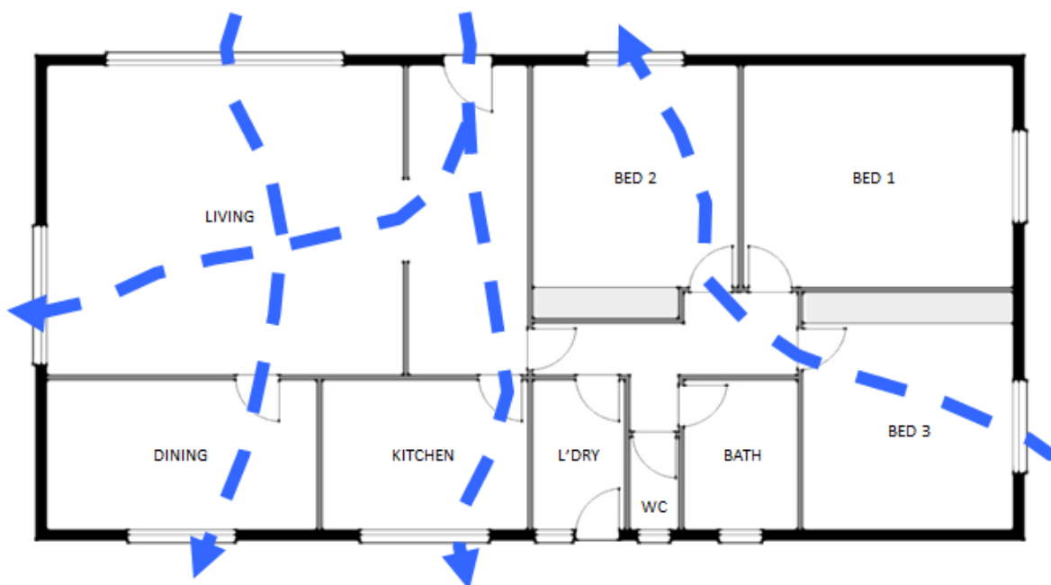
Figure 11.1 Cross flow ventilation
