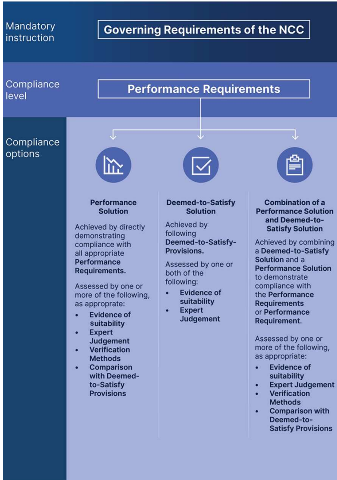
Figure C.1 Demonstrating compliance with the NCC
