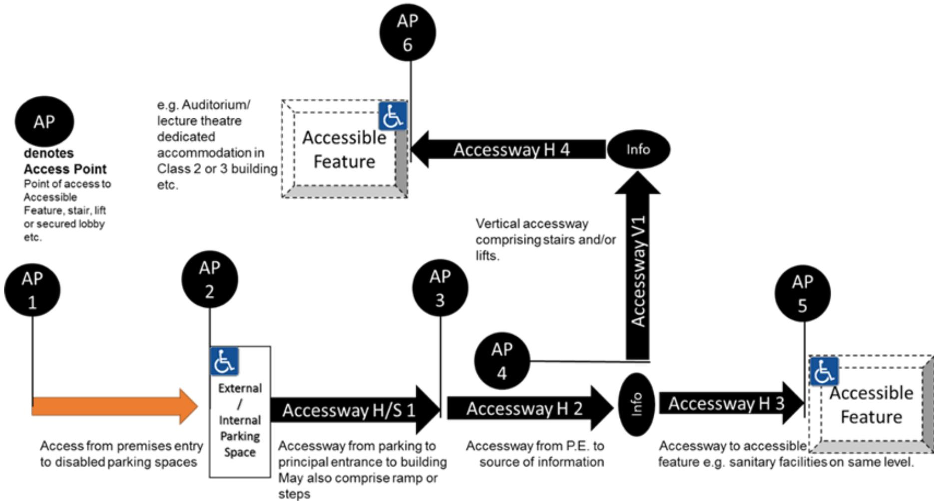
For the purpose of the accessway and accessible features model of Figure 4.1:
