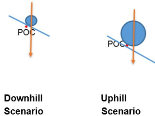
If the centre of gravity is outside of the point of contact (POC), as shown in Figure 5.1 and Figure 5.2, the wheelchair is at risk of tipping and therefore the ramp is not suitable.
