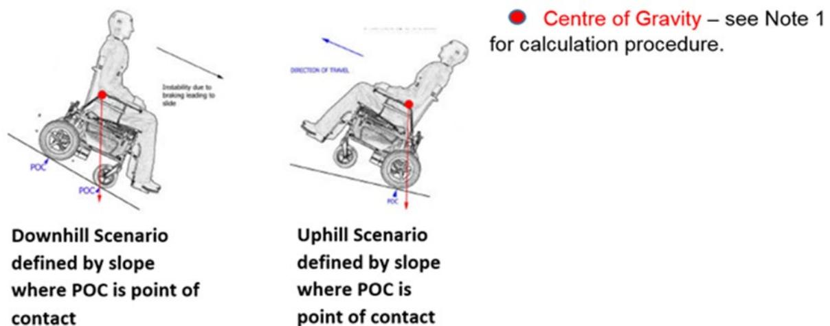
Note 1: Using the PWC model, draw in the vertical component of the force representing the distribution of the mass of the PWC and the user as shown in Figure 5.1.
