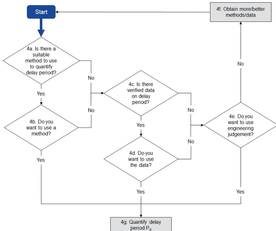
The following steps comprise the quantification of delay period as set out in Figure A.5.5.
