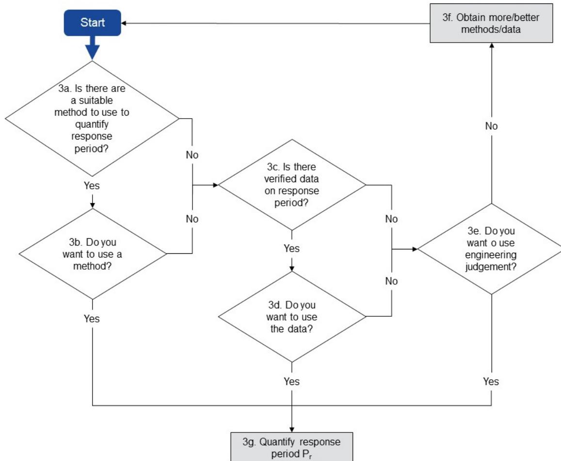
The following steps comprise the quantification of response period as set out in Figure A.5.4.
