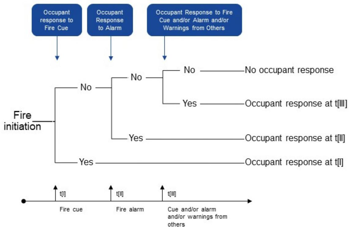
Each of the above four occupant detection response scenarios, as shown in Figure 3.1.3, should be combined separately with each of the fire scenarios identified in Figure 3.1.2.
