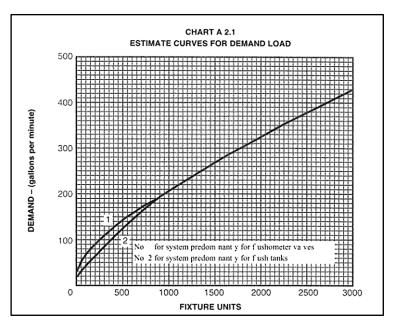
Figure 1 Estimate curve for design purposes <sup>9</sup>
