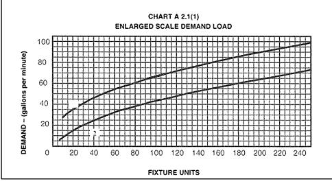
Figure 2 Enlarged scale demand load<sup>10</sup>
