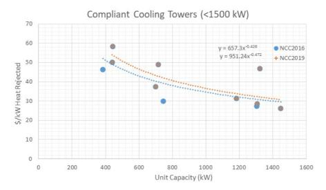
Figure 19: Cooling tower \$/kW comparison for NCC0216 and NCC2019.
