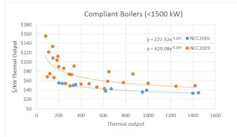
Figure 18: Comparison of compliant boilers for NCC2016 and NCC2019.
