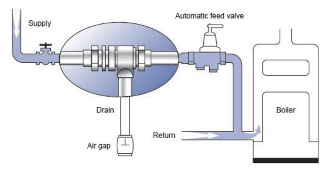
Figure 6.11 Dual check valve with atmospheric port—typical installation
