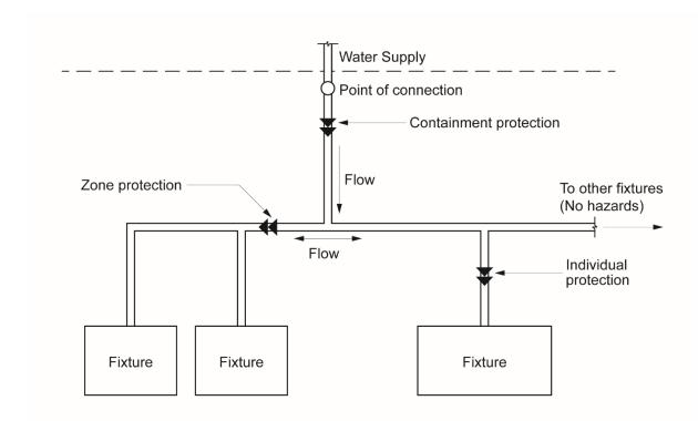
Figure 2.1 Individual, zone and containment protection
