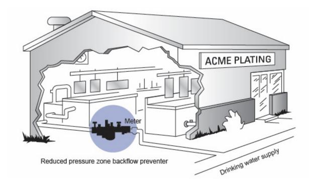
Figure 6.15 Reduced pressure zone device—typical installation (example 1)
