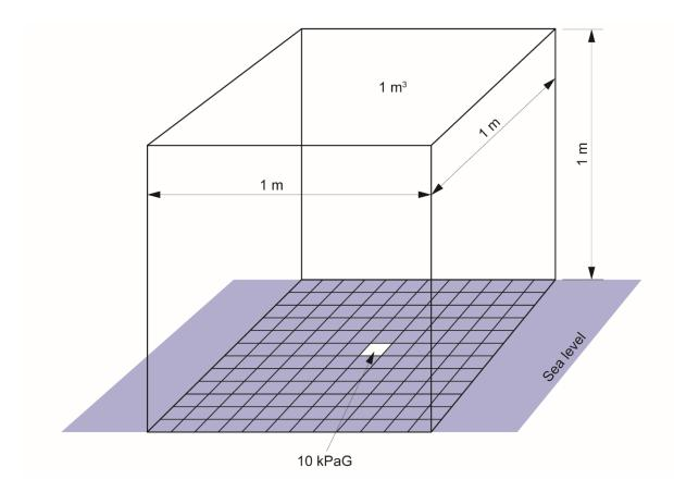
Figure 3.1 Pressure exerted by 1 metre of water at sea level
