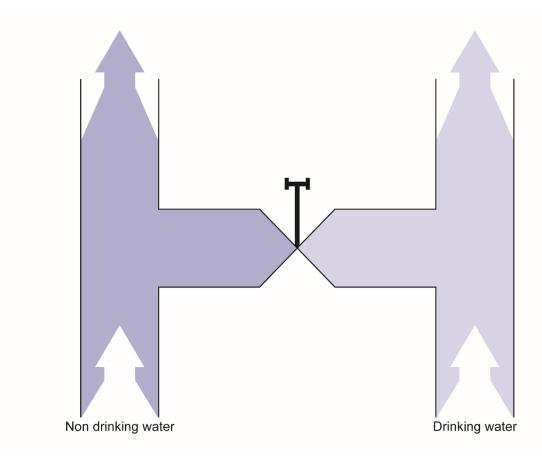
Figure 3.10 Valved connection between drinking water and non-drinking water
