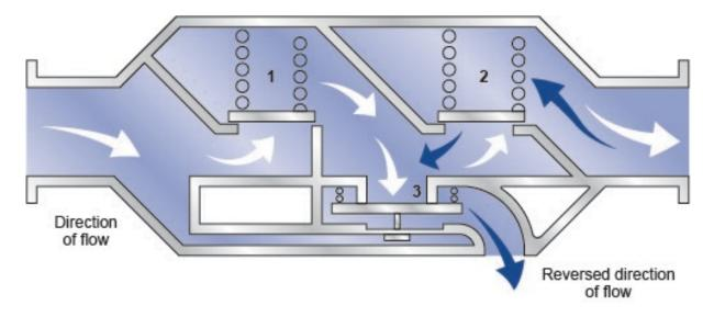
Figure 6.14 Reduced pressure zone device (RPZD)
