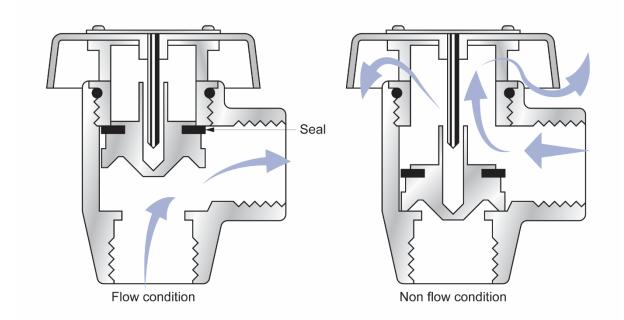
AVBs should be installed vertically and should not have any shutoffs downstream of the device. They should be installed at least 150 mm higher than the highest downstream outlet. Figure 6.4 shows the typical installation of an AVB. Note that no shutoff valve is installed downstream of the device that would otherwise keep the AVB under continuous pressure.
