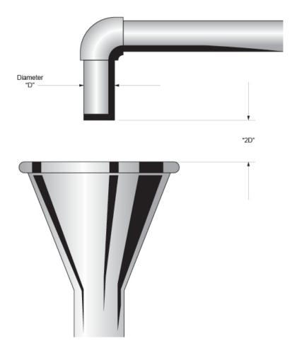
An air gap, although an extremely effective backflow preventer when used to prevent backsiphonage and backpressure conditions, may cause a corresponding loss of pressure to downstream outlets. Consequently, air gaps are primarily used at end of line services where reservoirs or storage tanks are desired.
