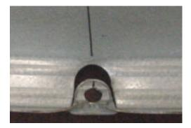
Figure 4.7 Stramit Batten failure mode
