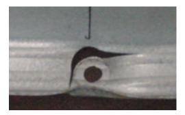
Figure 4.6 Stramit Batten failure mode
