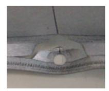
Figure 4.3 BHP batten static failure mode at the unsymmetric wider turned over edge
