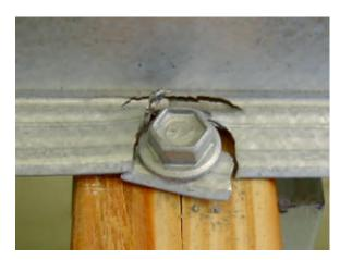
Figure 4.14 Batten failure in Cyclone Testing Station air-box test
