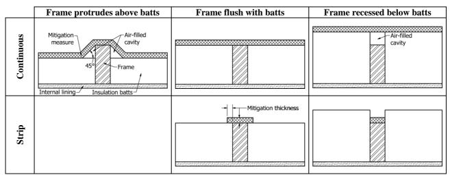
Figure 4: Examples that demonstrate how strip and continuous mitigation measures were applied for different combinations of batt and frame heights. Note that strip mitigation measures were not examined in cases where the frame protruded above the batts. These partial cross-sections are used to highlight the mitigation geometry and do not illustrate the full computational domain modelled in cases with mitigation measures, which were similar to those shown in Figure 2 and Figure 3.
