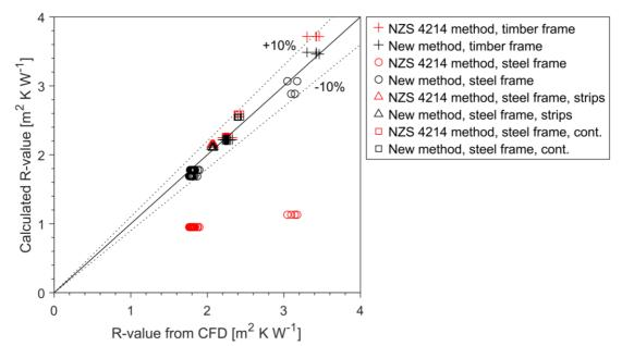
Figure 8: R-values calculated using the standard NZS 4214 method and the new method developed here (with separate 'timber only' and 'steel only' models), compared to values obtained through CFD simulations in the original thermal bridging study for the ABCB with thermal bridge mitigation options of strips or continuous layers of insulation added [5].
