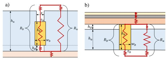
Figure 5: Partial cross-section of a thermally bridged (a) ceiling with battens oriented perpendicular to the joist, and (b) suspended floor, showing key parameters used in Equation 2.
