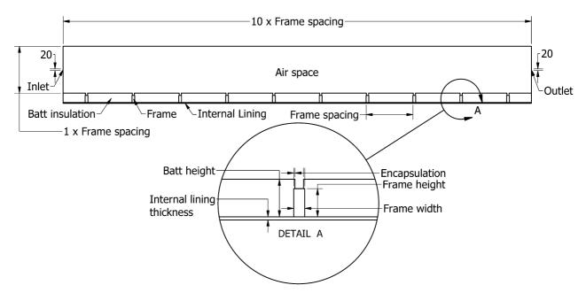
*Figure 2: Example of the two-dimensional computational domain developed for the CFD simulations of horizontal assemblies with top surfaces exposed to an air space.*
