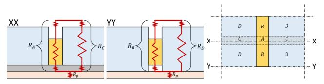
Figure 6 Example ceiling assembly showing two vertical cross-sections and a plan view indicating the heat flow paths and the areas through which they flow. Note that the batten has been made visible in the plan view diagram using dashed lines.
