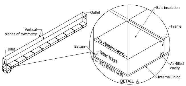
Figure 3: Example of the three-dimensional computational domain developed for CFD simulations of horizontal assemblies with battens. Note that a symmetry boundary condition was applied at the vertical plane that bisects the batten.
