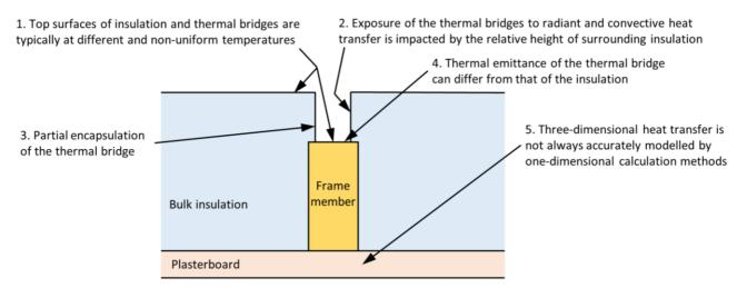
Figure 1: Factors that can contribute to the inaccuracy of the standard NZS 4214 calculation method when applied to ceilings and suspended floors. Numbers correspond to the sources of inaccuracy listed in the text above the figure.
