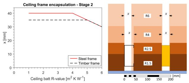
Figure 11: Alternative assumptions regarding the level of encapsulation of frame members by adjacent insulation. The dimension x represents the width of the gap between adjacent batts, above each frame member.
