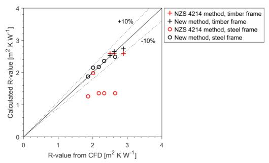
Figure 9: R-values calculated using the standard NZS 4214 method and new method developed here (with separate 'timber only' and 'steel only' models), compared to values obtained through CFD simulations in the study completed for NASH [6].
