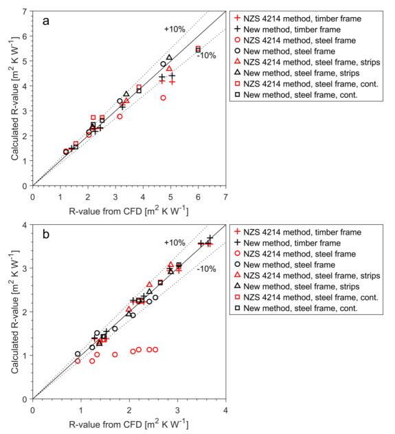
Figure 10: R-values calculated using the standard NZS 4214 method or new method developed here (with separate 'timber only' and 'steel only' models), compared to values obtained through CFD simulations in Stage 1 of this study [7], for: (a) ceilings, and (b) suspended floors.
