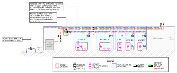
Figure 2 Single user amenities building schematic for Scenario 1 – Existing Configuration noting Required Works to Facilitate Monitoring
