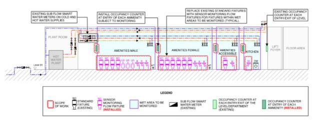
Figure 8 Multiple user amenities building schematic for Scenario 3 – Existing Configuration noting Required Works to Facilitate Monitoring
