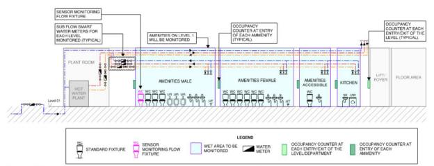
Figure 5 Multiple user amenities building schematic illustrating potential monitoring components to be identified during the Preliminary Investigation Stage
