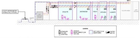
Figure 4 Single user amenities building schematic for Scenario 3 – Existing Configuration Suitable for Monitoring
