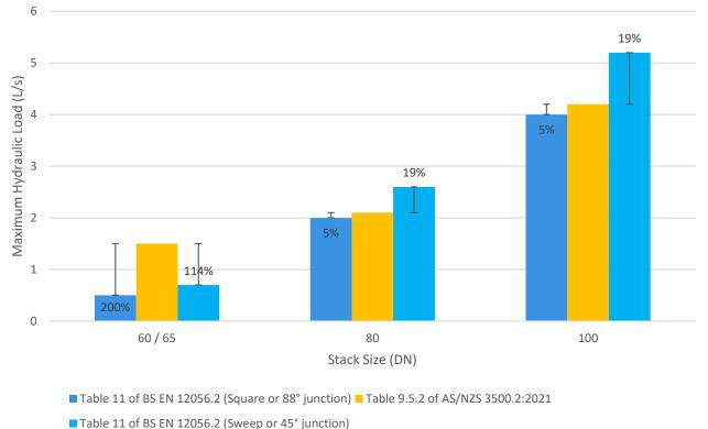
Figure 8: Percentage Difference between Stack Capacities reported in Table 9.5.2 of *AS/NZS 3500.2:2021* and Table 11 of BS EN 12056.2 Square or 88° junction, and Sweep or 45° junction
