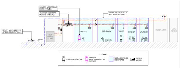
Figure 1 Single user amenities building schematic illustrating potential monitoring components to be identified during the Preliminary Investigation Stage
