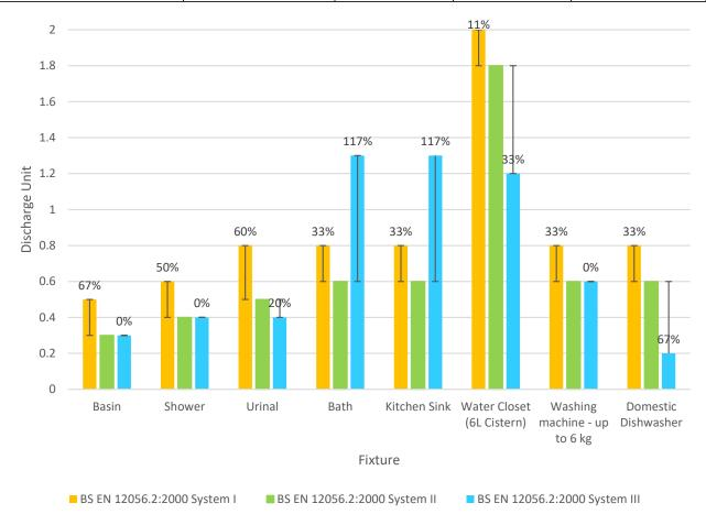
Figure 13: Variation in Discharge Unit of each Fixture for System I to III with Percentage Differences between System I and System I & III
