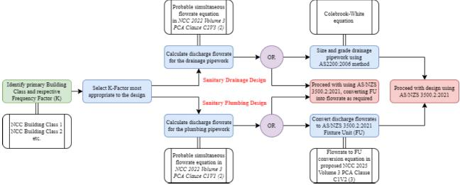
Figure 25: Verification Method Workflow for Sanitary Plumbing and Drainage Designs
