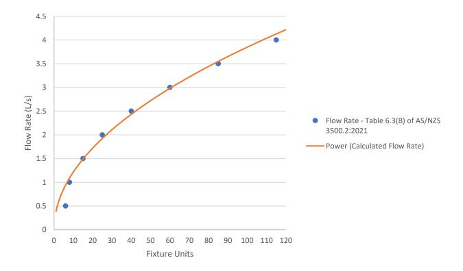
Figure 4: Fixture Units versus Flow rate for data provided in Table 6.3(B) of *AS/NZS 3500.2:2021* and calculated flow rate using 'Fixture Unit to Flow Rate' Formula
