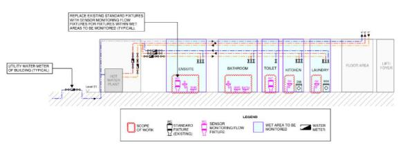
Figure 3 Single user amenities building schematic for Scenario 2 – Existing Configuration Noting Required Works to Facilitate Monitoring
