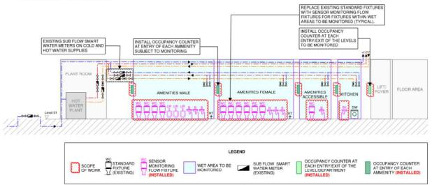
Figure 7 Multiple user amenities building schematic for Scenario 2 – Existing Configuration noting Required Works to Facilitate Monitoring
