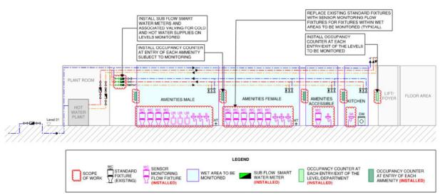
Figure 6 Multiple user amenities building schematic for Scenario 1 – Existing Configuration noting Required Works to Facilitate Monitoring
