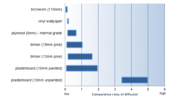
The driving force for adsorption is a difference in vapour pressure across a material or between spaces.
