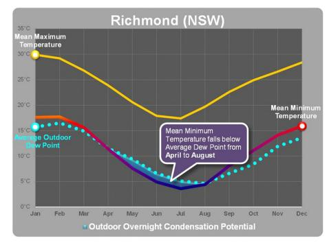
Figure 3.24 Comparison of monthly mean minimum temperatures and average dew points (outdoor overnight condensation potential)
