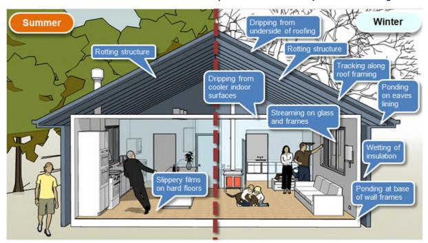
Figure 3.17 Some risks from condensation in the occupied and interstitial space of a building
