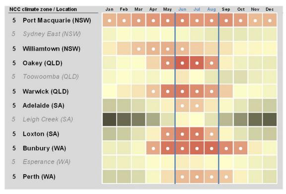
Figure 3.20 uses BOM data to compare the mean minimum temperature in each month with the average dew point temperature, based on 9am and 3pm data, for that month. Where the mean minimum temperature falls on or below the average dew point, the table
