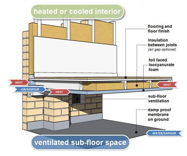
Figure 4.15 Suspended timber framed floor with summertime risk of inward vapour drive
