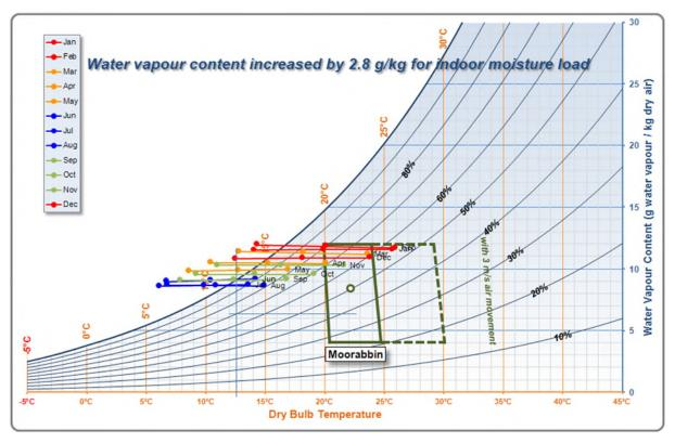
Figure D.11 Water vapour content values adjusted for indoor load – Canberra (ACT)
