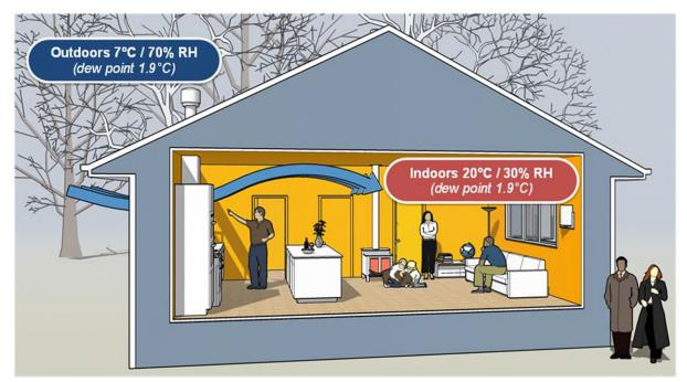
Figure 3.11 Warmer indoor temperature lowering RH of outdoor air from outdoors
