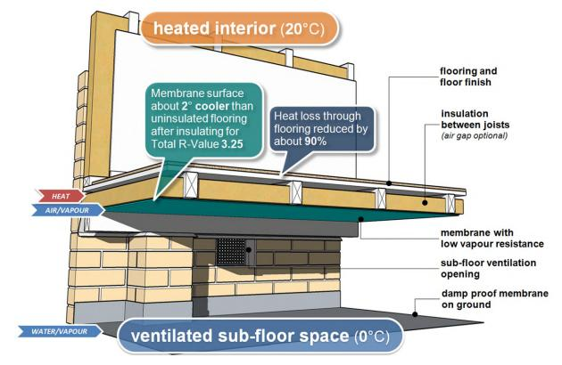
Figure 4.5 Suspended timber framed floor - insulated between joists (alpine/cold climate)
