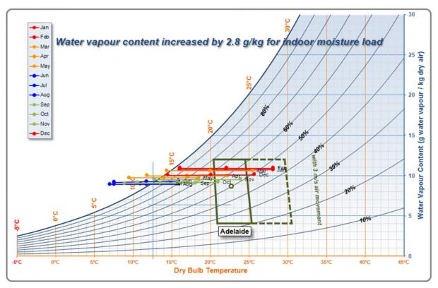
Figure D.9 Water vapour content values adjusted for indoor load –Mascot, Sydney (NSW)
