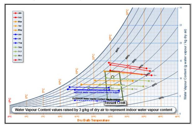
Figure 3.35 Water vapour content values adjusted for indoor load – Tennant Creek (NT)
