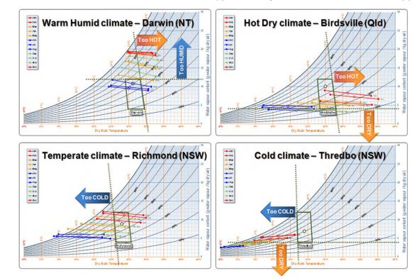
Figure 3.29 Characteristics of the four basic climate types (enlarged versions are located in Appendix D)
