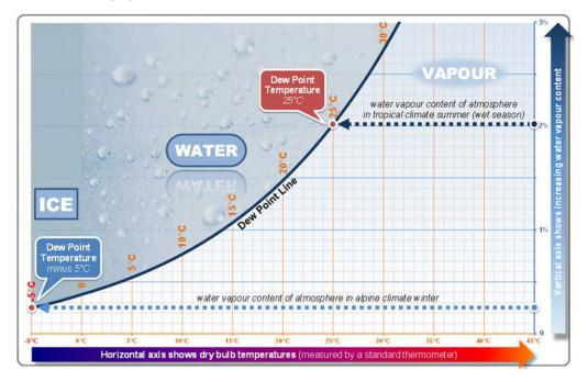
The key feature of the chart is the diagonal curve which separates the gridded vapour zone on the right from the ice and water zones on the upper left. The intersection of any vertical temperature line with the curve marks the saturation limit for that temperature. Reading across the chart, to the vertical axis, reveals the water vapour content of the atmosphere at that saturation limit (as a percentage by mass of the atmosphere in this version of the chart).
