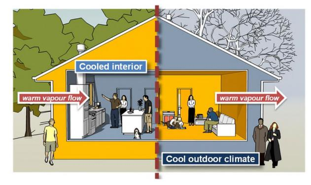
Figure 3.5 Critical temperatures driven by artificial cooling indoors or by the climate outdoors
