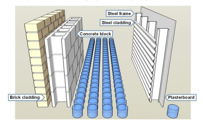
Figure 3.16 Comparative safe moisture storage capacity of masonry and light framed walls
