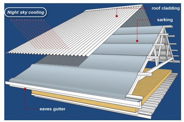
Figure 4.7 Draining condensate formed on the underside of roof cladding
