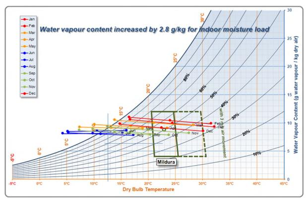
Figure D.7 Water vapour content values adjusted for indoor load – Perth (WA)
