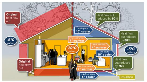
The outward heat flows through the roof and wall on the left side of Figure 3.6 also demonstrate why an uninsulated building would have warmer cavities and air spaces. These benefits will last only while massive heat loss outwards from the warm interior can be sustained.
