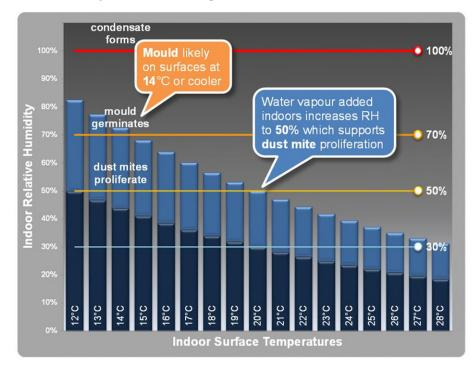
Figure 3.12 Warmer indoor temperature lowering RH of outdoor air from outdoors
