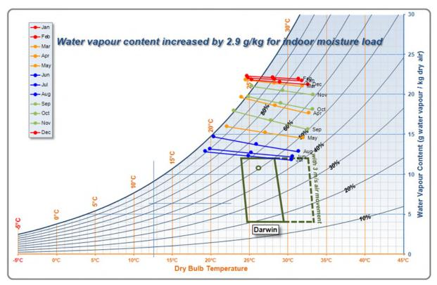
Figure D.3 Water vapour content values adjusted for indoor load – Townsville (Qld)
