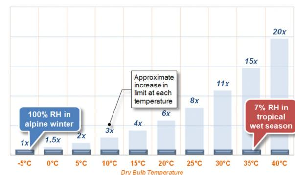
Figure 3.9 Approximate increases in water vapour limits rising with temperature Note: When the amount of water vapour is fixed, the RH falls as the temperature rises
