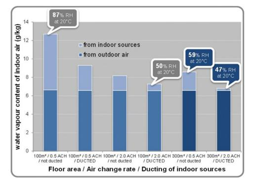
Figure 3.32 Impact of indoor volume, air change rate and ducting of sources on indoor humidity
