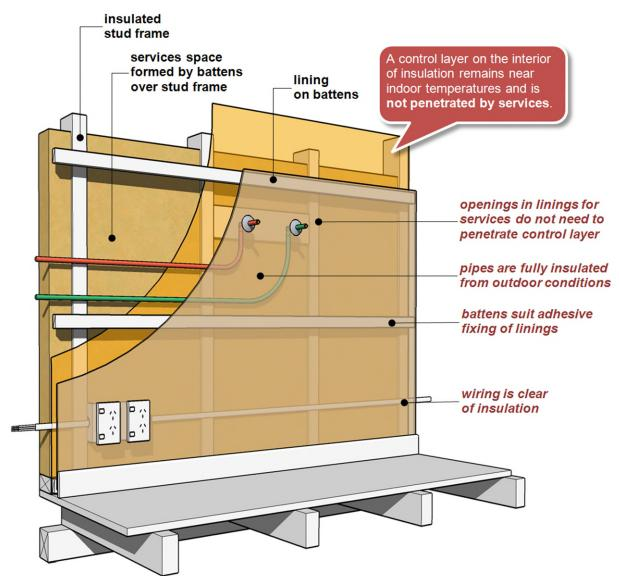
Emphasising the importance of effective air control, the British Standard BS 5250:2011+A1:2016, Annex G, advises that a dedicated space for the installation of services should be formed behind interior surface finishes or linings. This will allow an air control layer to be formed on the interior side of wall insulation without penetrations for services, as illustrated in Figure 4.12.
