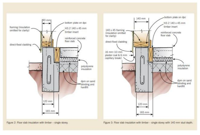
Figure 17. External wall thickness definitions as defined by Ian Cox-Smith (BRANZ) in Build Magazine (page 105, BUILD June/July 2007 – accessed: https://www.buildmagazine.org.nz/assets/PDF/B100-103-InsulateSlab.pdf)
