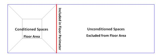
Figure 19 Floor Area and Floor Perimeter for Conditioned Spaces connected to Unconditioned Spaces
