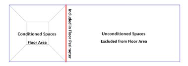
Figure 1 Floor Area and Floor Perimeter for Conditioned Spaces connected to Unconditioned Spaces
