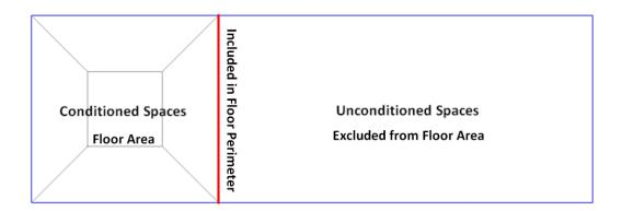
Figure 13 Floor Area and Floor Perimeter for Conditioned Spaces connected to Unconditioned Spaces
