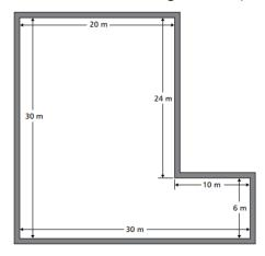
Figure 2 Example 3.4 in CIBSE Section 3.5 indicating the floor area and the floor perimeter is calculated from calculated from the interior surface of the external wall surrounding the floor
