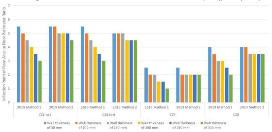
Figure 5 Inflection Points of Floor Area to Floor Perimeter Ratio (Soil Type - Sand or Gravel)
