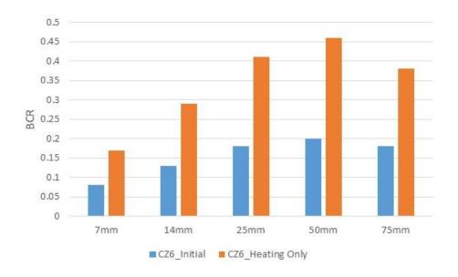
Figure 11 BCR Results for Motel Models in CZ6 (Sensitivity Analysis for Edge Insulation)
