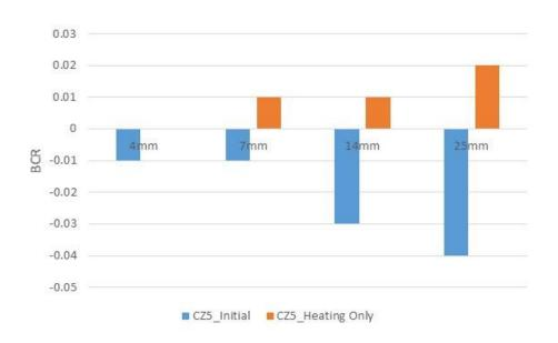
Figure 10 BCR Results for Office Model in CZ5 (Sensitivity Analysis for Edge Insulation)
