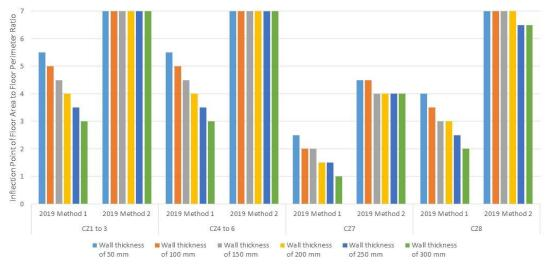
Figure 6 Inflection Points of Floor Area to Floor Perimeter Ratio (Soil Type - Homogeneous Rock)
