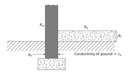
Total equivalent thickness of floor:  $d_{ef} = d_w + \lambda_g (R_{si} + R_f + R_{se})$
