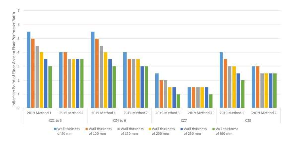
Figure 4 Inflection Points of Floor Area to Floor Perimeter Ratio (Soil Type - Clay or Silt)
