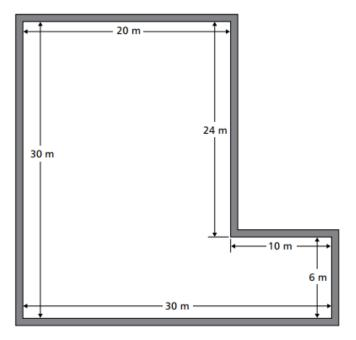
Figure 20 Example 3.4 in CIBSE Section 3.5 indicating the floor area and the floor perimeter is calculated from calculated from the interior surface of the external wall surrounding the floor
