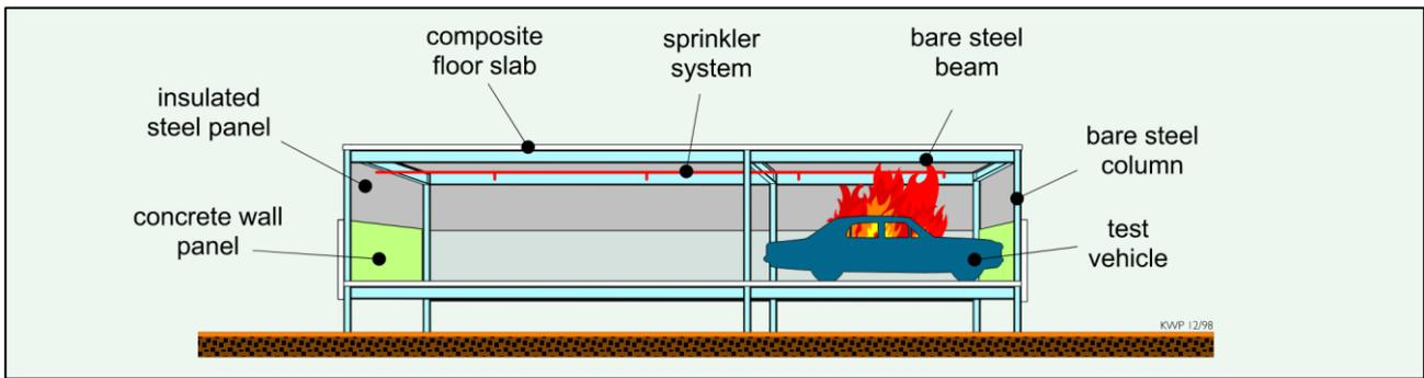
**Figure 8: Isometric section drawing showing closed carpark experiment arrangement. Reproduced from [49]. © BHP.**
