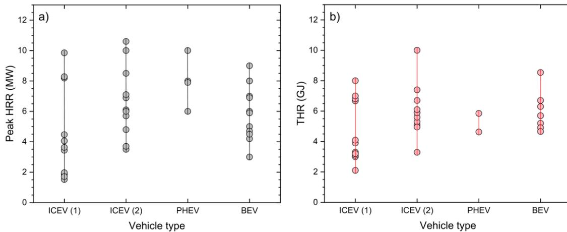
**Figure 37: a) Peak HRR and b) Total Heat Released for ICEVs, PHEVs and BEVs. 'ICEV (1)' represents vehicles manufactured before 2000, whereas 'ICEV (2)' represents vehicles manufactures after 2000. Reproduced from [160].**
