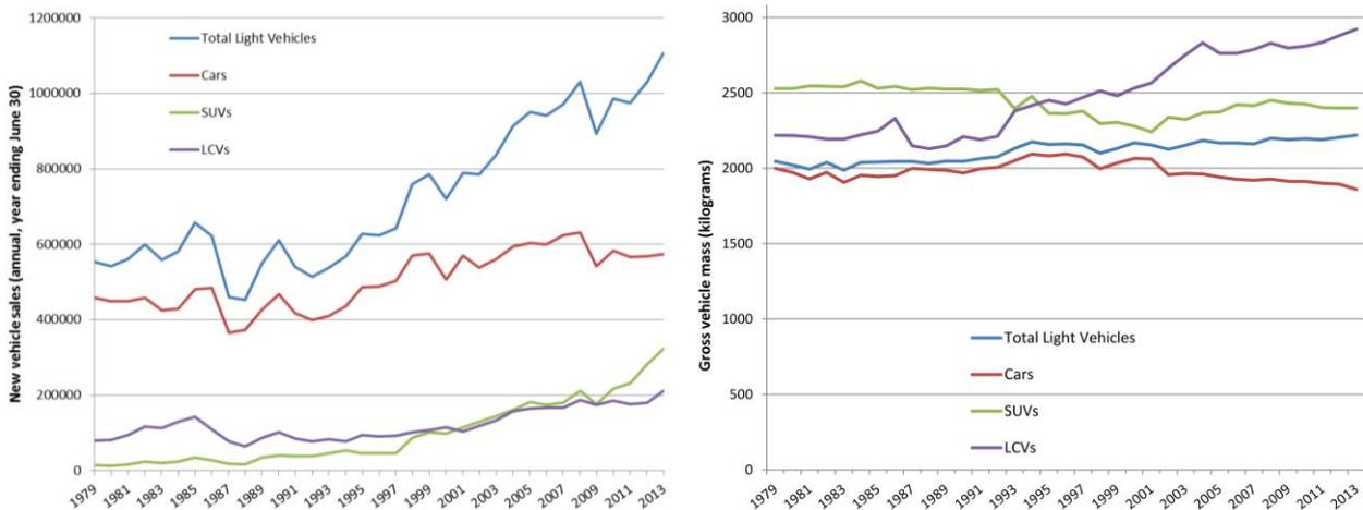
**Figure 26: Left: New light vehicle sales in Australia. Right: Average Gross Vehicle Mass (GVM) for new light vehicles purchased in Australia. Data from 1979-2013. Reproduced from [128].**
