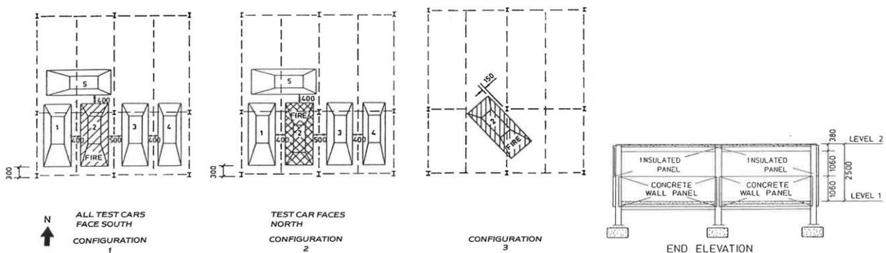
**Figure 9: Plan and elevation drawings showing test building. Reproduced from [43].**
