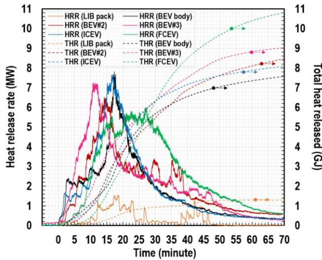
Figure 36: Comparison of the HRR from a BEV, ICEV and Hydrogen FCEV. Reproduced from [159].
