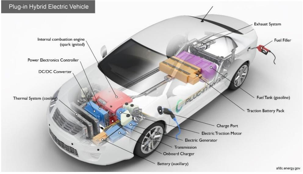
Figure 30: Typical plug-in hybrid electric vehicle (PHEV) layout. © Alternative Fuels Data Center.
