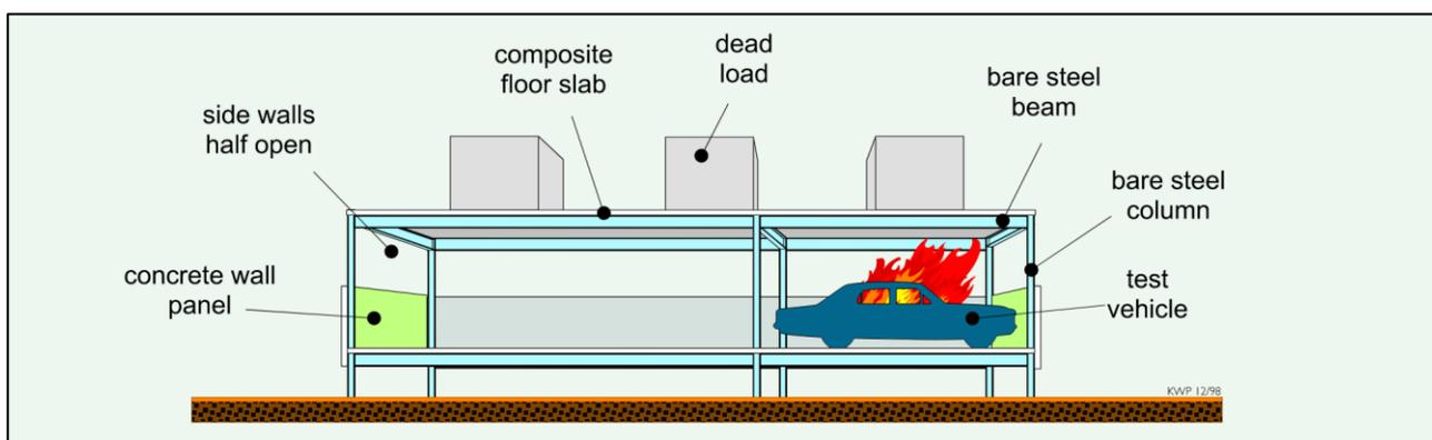
**Figure 5: Isometric section drawing showing open-deck carpark experiment arrangement. Reproduced from [49]. © BHP.**
