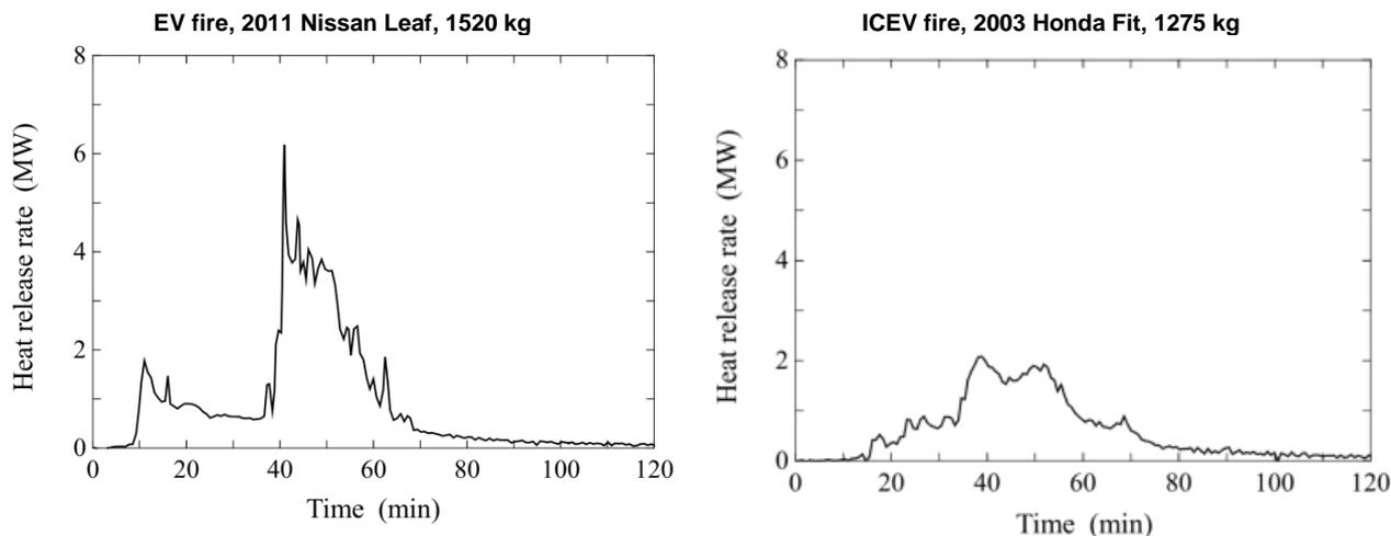
**Figure 34: Comparison of the HRR from EV and ICEV tests from two manufacturers. Reproduced from [156].**
