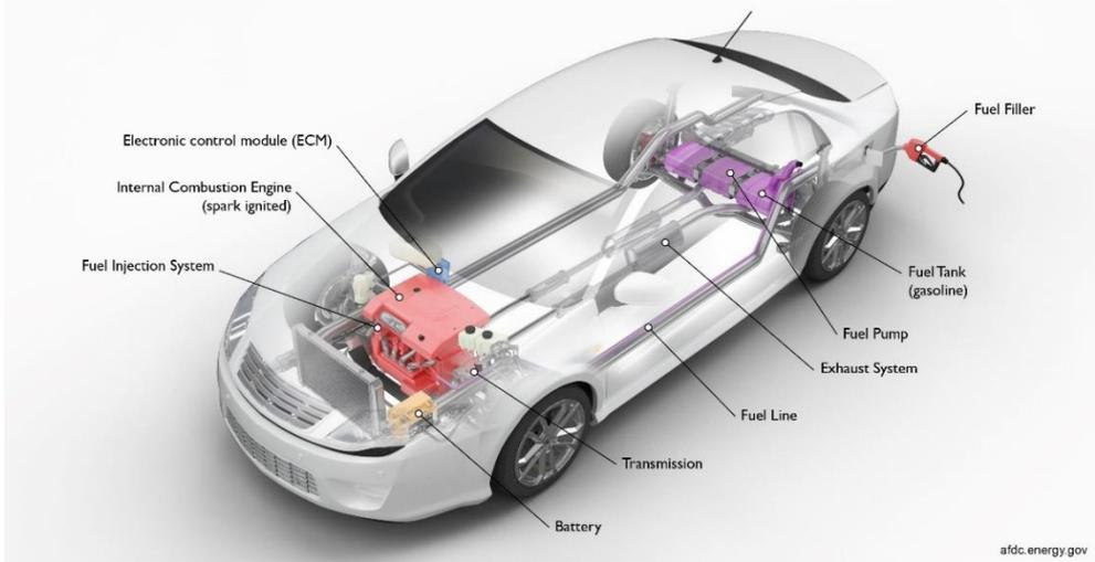
Figure 27: Typical petrol or diesel powered internal combustion engine vehicle (ICEV). © Alternative Fuels Data Center.
