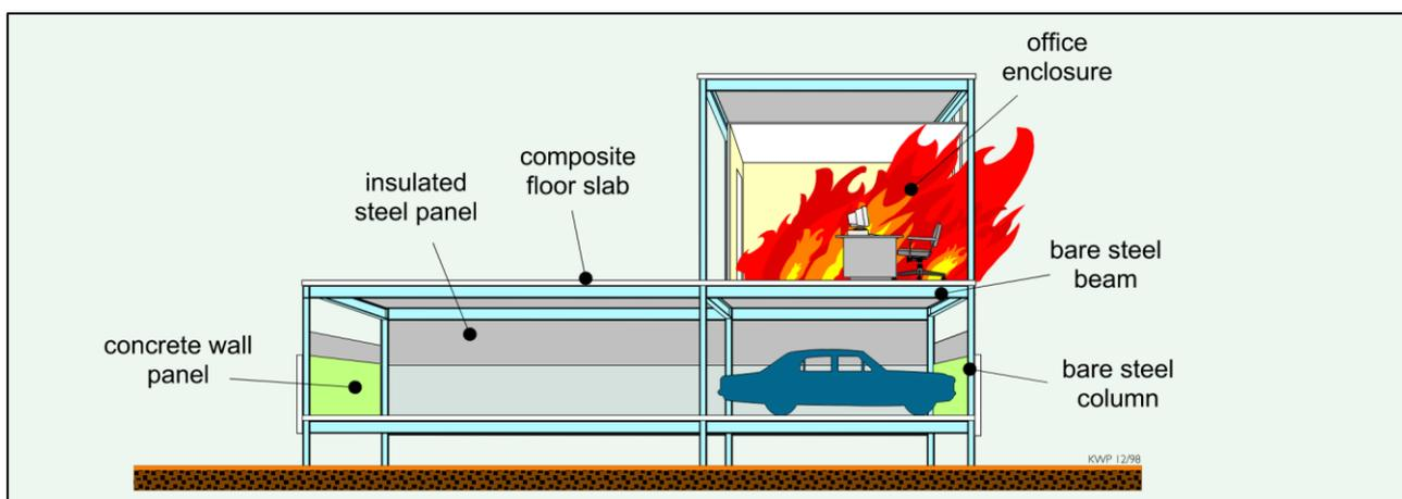
**Figure 12: Isometric section drawing showing experiment arrangement with fire originating in another part of the building. Reproduced from [49]. © BHP.**
