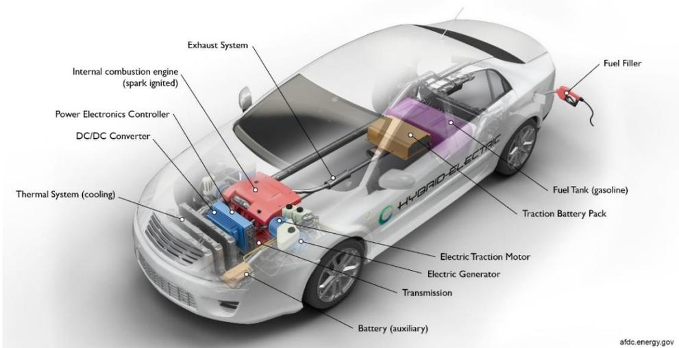
Figure 29: Typical hybrid electric vehicle (HEV) layout. © Alternative Fuels Data Center.
