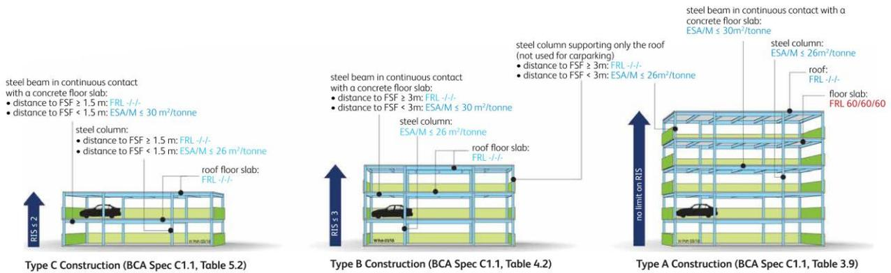
**Figure 1: Structural FRL requirements for carparks within the NCC 2019. Reproduced from [6]. © Liberty Steel.**
