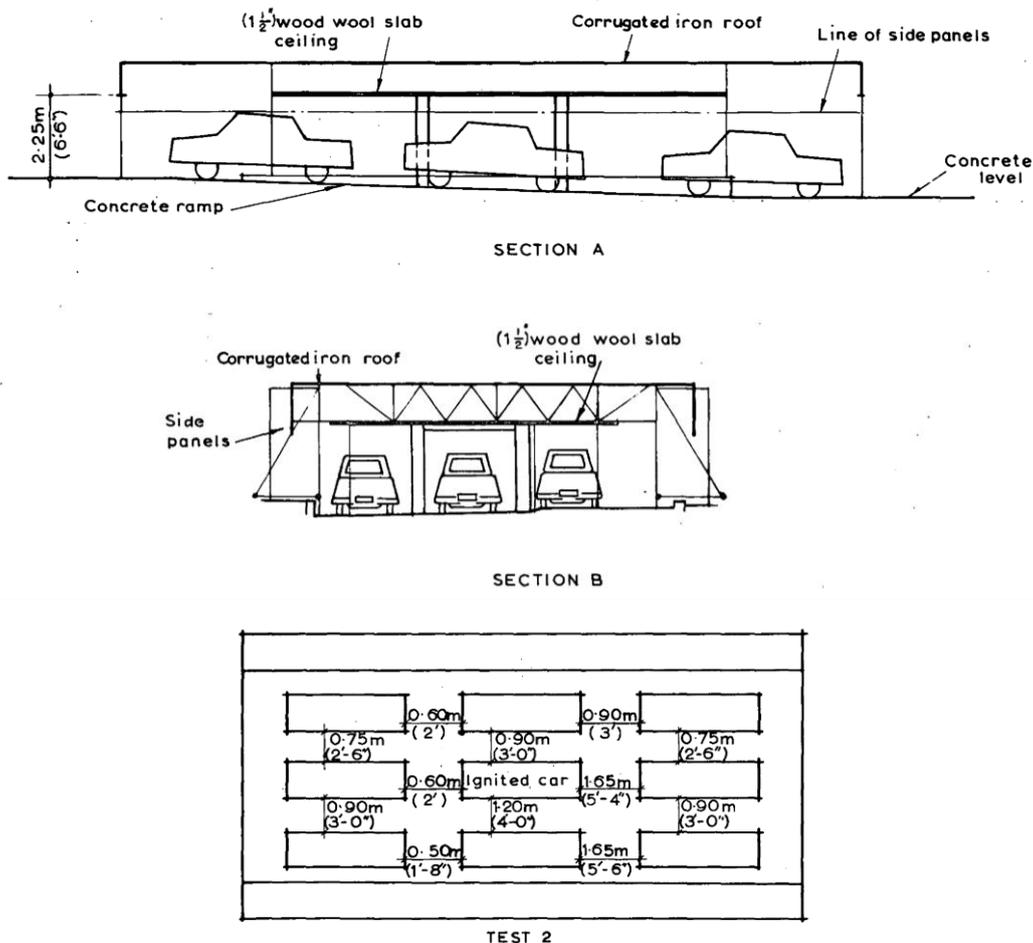
**Figure 4: Section and plan views of the UK JFRO carpark experiments. Reproduced from [35].**
