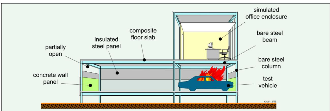
Figure 10: Isometric section drawing showing partially open carpark arrangement. Reproduced from [49]. © BHP.
