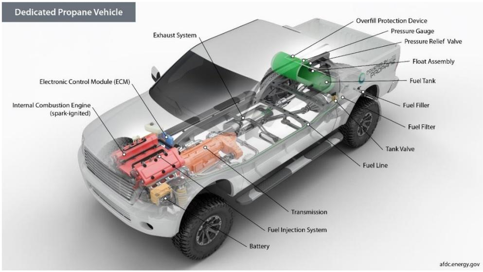
Figure 32: Typical liquefied petroleum gas (LPG) vehicle layout. © Alternative Fuels Data Center.
