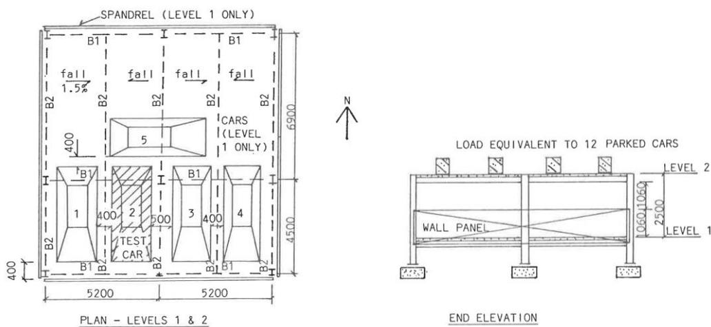
**Figure 6: Plan and elevation drawings showing test building. Reproduced from [42]. © BHP**
