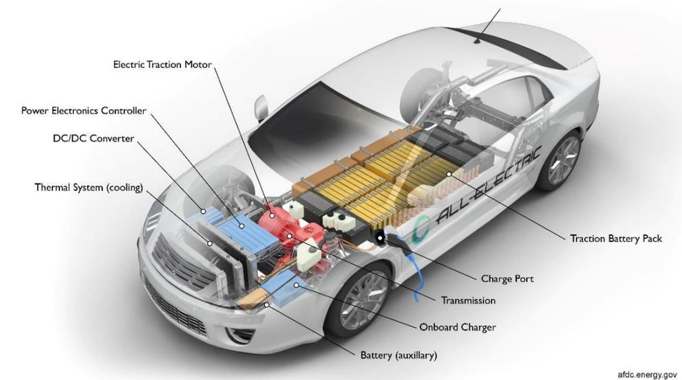
Figure 28: Typical battery electric vehicle (BEV) layout. © Alternative Fuels Data Center.
