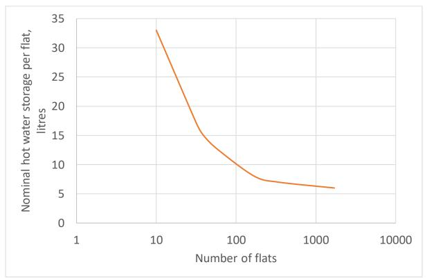
Figure 11: Estimated minimum hot water storage requirement per dwelling for central hot water systems in Class 2 buildings.
