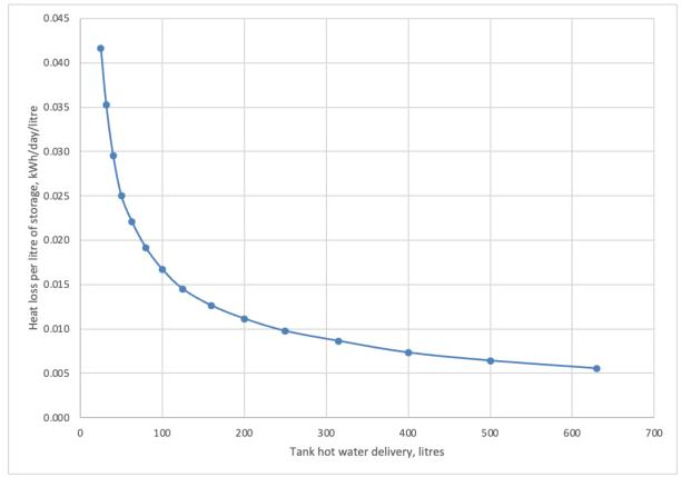
Figure 10: Heat loss per litre of storage as specified in AS/NZS4692.2 Source: Author calculations based on AS/NZS4692.2 permitted heat loss values for mains pressure units.
