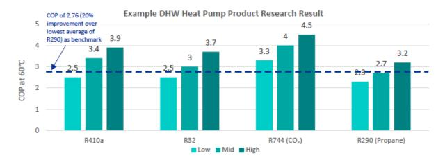
**Figure 9: Benchmark COP performance of a range of heat pump systems** Figure notes: Source is Figure 7 from NatHERS DHW and HVAC Methodology for Apartment Shared Services, Bridgeford Group (V1.4, 24 July 2023)
