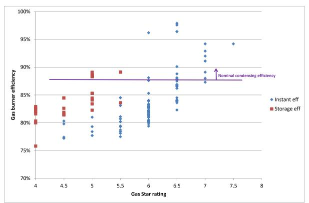
Figure 6: Gas star rating versus burner efficiency for residential gas hot water systems
