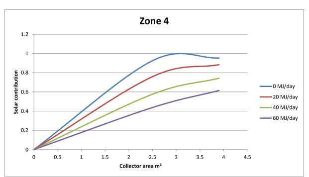
Figure 12: Change in solar contribution with changes in collector area for different hot water demands
