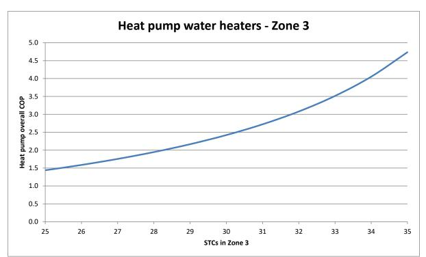
Figure 7: STCs versus overall system COP for heat pump water heaters in AS/NZS4234 Zone 3
