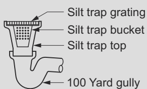
SILT TRAP ASSEMBLY
