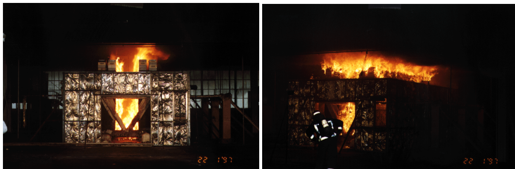
FIGURE 6.8 TEST 4 UNSPRINKLERED SHOE STORAGE
