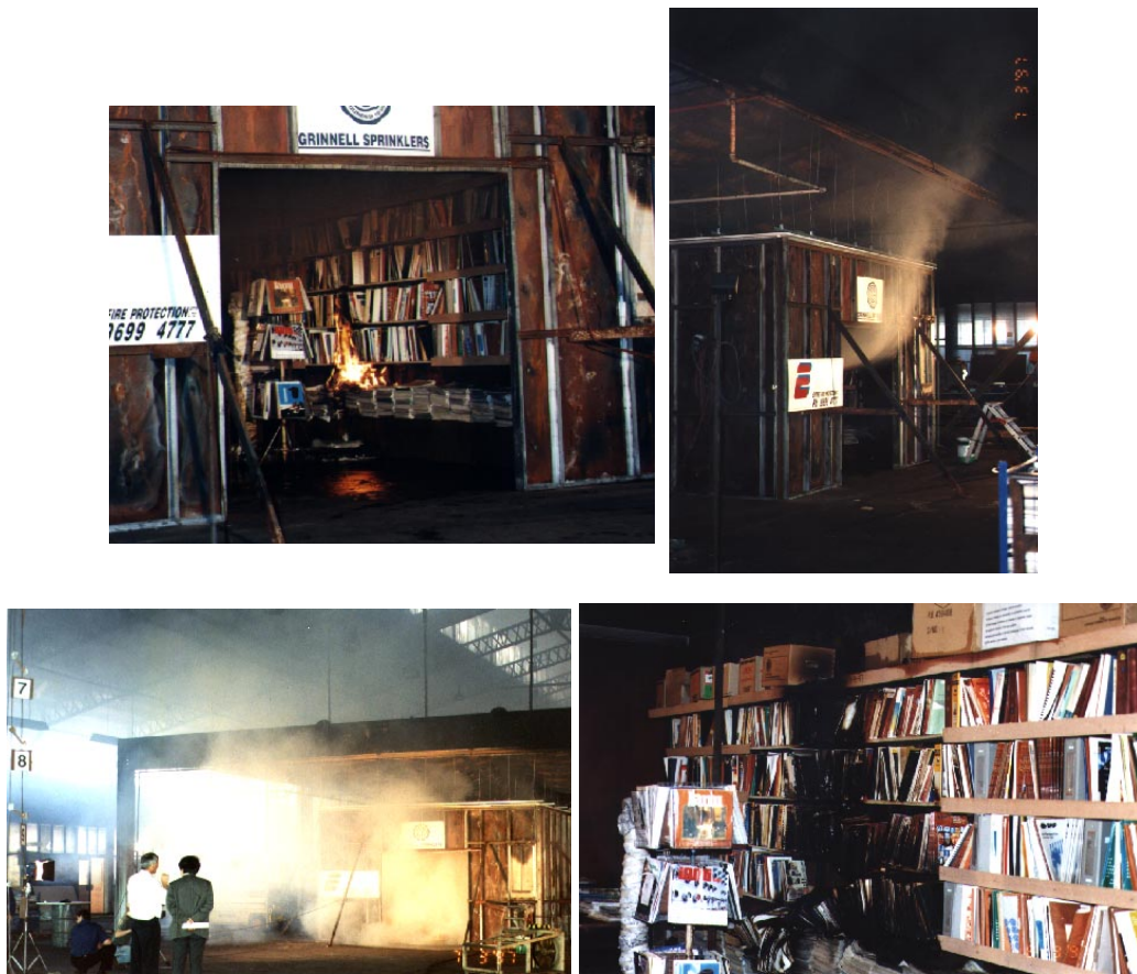
FIGURE 6.10 TESTS 10-11 SPRINKLERED BOOK SHOP
