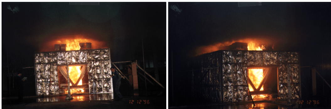
FIGURE 6.7 TEST 3 SPRINKLERED SHOE STORAGE
