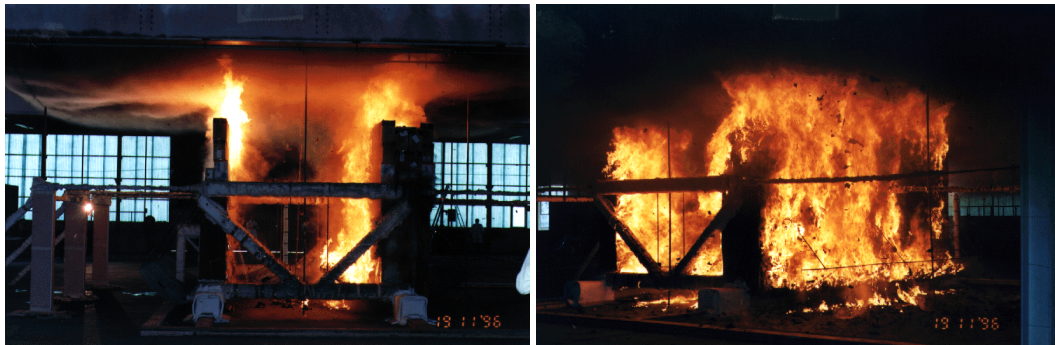
FIGURE 6.6 TEST 2 UNSPRINKLERED TOY SHOP
