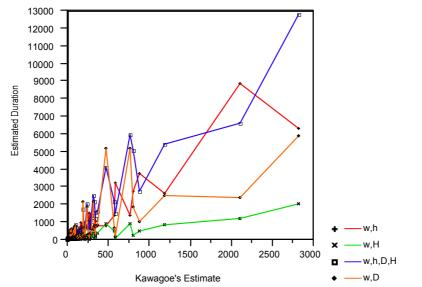
Figure 20 Comparison of Various Fire Duration Estimates (minutes) with Kawagoe's Estimate for the Range of Enclosure and Opening Dimensions for Project 3
