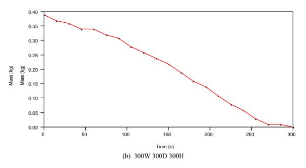
Figure 6 Typical Reduction in Fuel Mass with Time - Trays of Liquid Fuel
