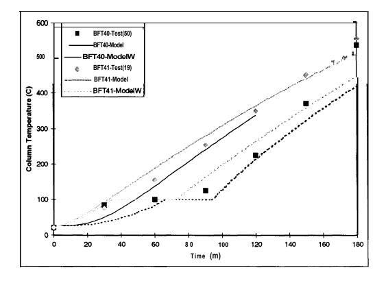
FIGURE 6. STEEL COLUMN TEMPERATURES.
