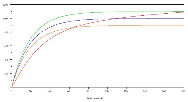
Figure 14 Comparison of Resulting Element Temperatures for Constant 900, 1000 and 1100°C and Standard Temperature-Time Regimes in Enclosure for StrucElem 1
