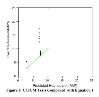
Tests conducted at VUT in an enclosure 5.4 m deep by 3.6 m wide by 2.4 m high with two opening sizes 3.16 m wide by 1.67 m high and 2.4 m wide and 1.5 m high resulted in nominal average heat outputs of 18.0, 19.4 and 24.7 MW for the first and 19.4, 20.9 and 20.9 MW for the second compared with Equation 1 estimates of 7.8 and 10.7 MW. Thus the measured values are from about two to three times the estimated values.
