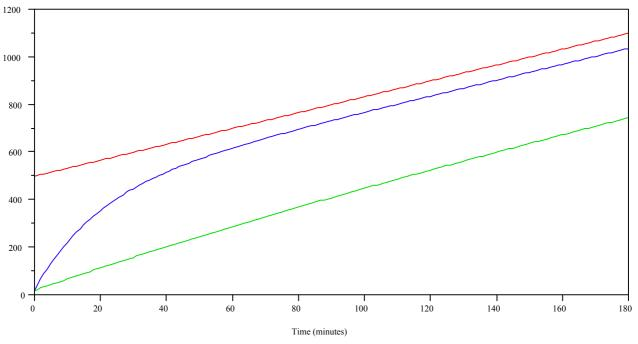
Figure 8 Temperature Enclosure and Resulting Element Temperature - Time Relationships
