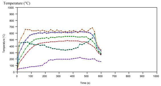
300 mm wide, 1500 mm deep, 200 mm high, wall material = steel, x = 1000 mm extra thermocouple 20 mm from floor, ??? mm from rear of enclosure on centreline arature (°C)
