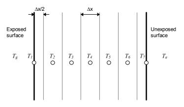
FIGURE 1. SUBDIVISION OF A BARRIER PANEL
