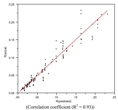
Figure 18 Scatter Diagram of Actual and Predicted Average Mass Loss Rate
