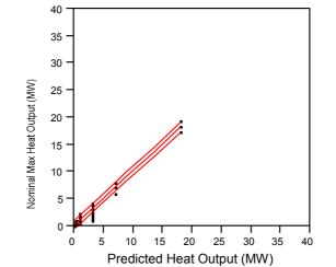
Figure 12 w/W = 1, Correlation of Equation 4 with Test Data
