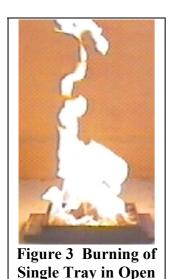
When burned in the open the fuel burned on all sides of the tray with the flames covering the entire tray. The flames were generally symmetrical and central above the tray (Figure 3).
