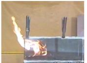
(a) Flames from front of **front tray** shortly after ignition - flames rise mainly from front edge of tray, travel back and up, and then largely forward and out of the enclosure
