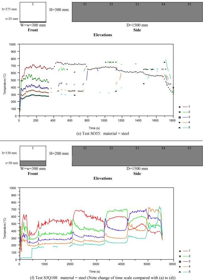
(f) Test S3Q108: material = steel (Note change of time scale compared with (a) to (d)) Figure 14 Examples of Temperature - Time Curves for Various Enclosure Configurations (continued)
