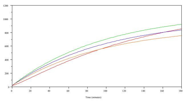
Figure 15 Comparison of Resulting Element Temperatures for Constant 900, 1000 and 1100°C and Standard Temperature-Time Regimes in Enclosure for StrucElem 2
