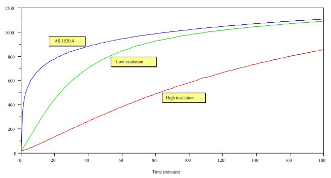
Figure 10 Standard Temperature-Time Response in Enclosure and Resulting Element Temperature - Time Relationships
