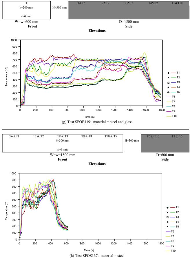
Figure 14 Examples of Temperature - Time Curves for Various Enclosure Configurations (continued)
