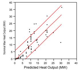
Figure 13 w/W < 1, Correlation of Equation 5 with Test Data
