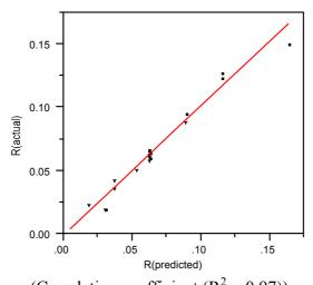
(Correlation coefficient ( $R^2 = 0.97$ )) Figure 21 Scatter Diagram of Actual and Predicted Average Mass Loss Rate
