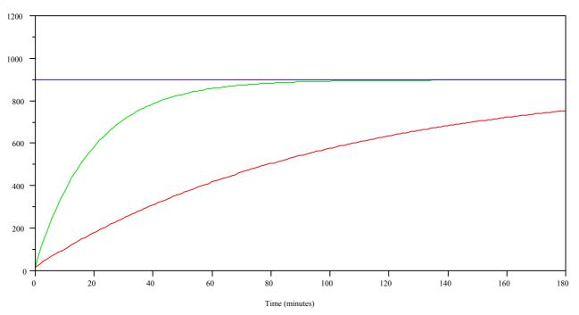
Figure 13 Constant 900°C Temperature-Time Response in Enclosure and Resulting Element Temperature - Time Relationships
