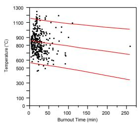
Figure 25 Correlation of Maximum Temperature with Burnout Time
