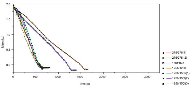
Figure 12 Variation in Fuel Mass During Tests in Enclosure 300 mm Wide, 1500 mm Long and 300 mm High
