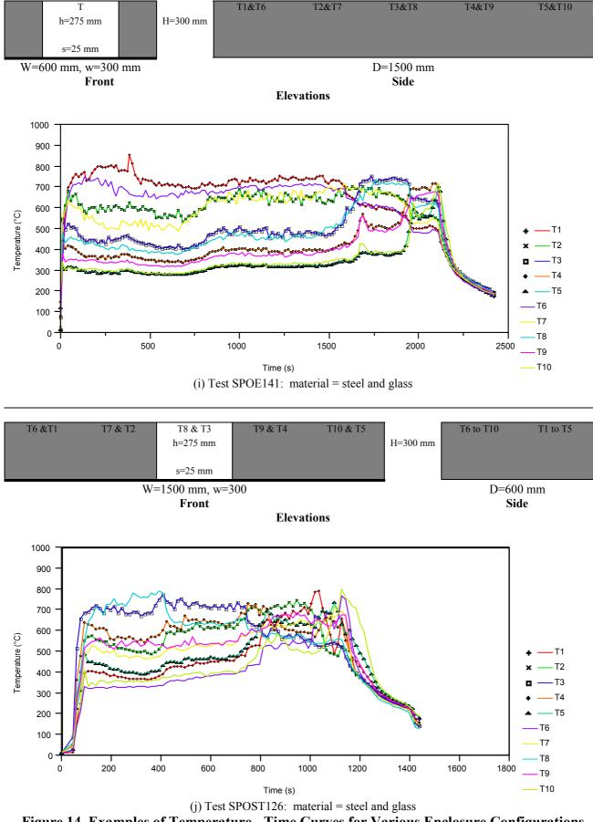
Figure 14 Examples of Temperature - Time Curves for Various Enclosure Configurations (continued)
