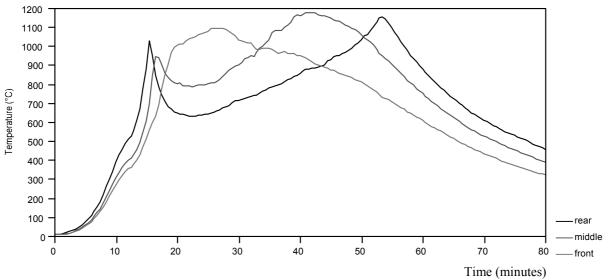
Figure 2 Temperature-Time Relationships for Three Cross-sections in an Enclosure 5.6 m Wide, 22.9 m Deep and 2.8 m High (Ignition at Rear)
