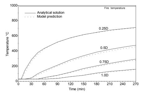
The results are shown in Figure E1 at quarter sections along the wall cross-section.
