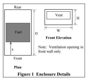
The following terminology and nomenclature is used for the clear internal dimensions of the enclosure (Figure 1):
