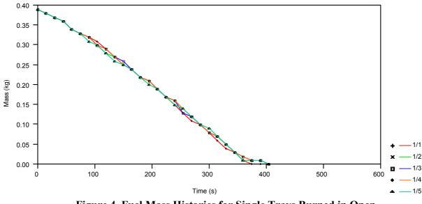
Figure 4 Fuel Mass Histories for Single Trays Burned in Open
