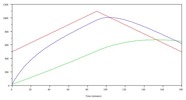
Figure 9 Temperature Enclosure and Resulting Element Temperature - Time Relationships
