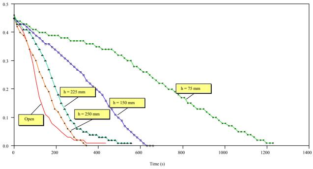
Figure 2 Reduction of Fuel Mass with Time for Wooden Cribs in the Open and in Enclosures with Opening Height as Shown
