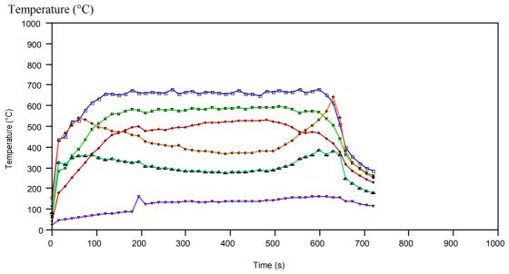
300 mm wide, 1500 mm deep, 200 mm high, wall material = steel, x = 800 mm extra thermocouple 20 mm from floor, ??? mm from rear of enclosure on centreline
