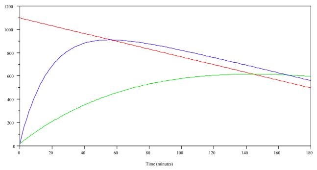
Figure 7 Temperature Enclosure and Resulting Element Temperature - Time Relationships
