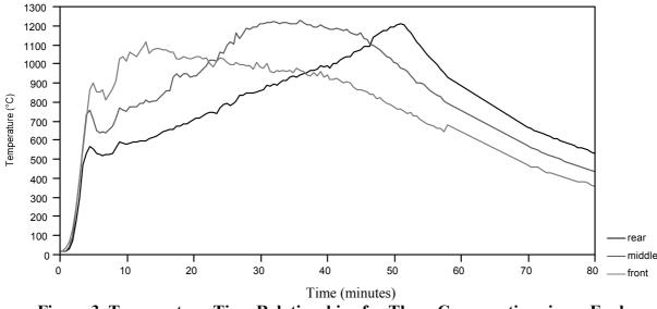
Figure 3 Temperature-Time Relationships for Three Cross-sections in an Enclosure 5.6 m Wide, 22.9 m Deep and 2.8 m High (Simultaneous Ignition)
