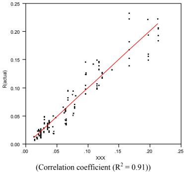
Figure 16 Scatter Diagram of Actual and Predicted Average Mass Loss Rate
