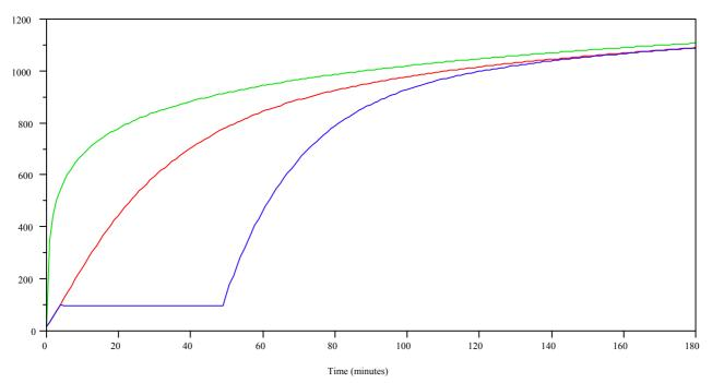
Figure 11 Standard Temperature-Time Response in Enclosure and Resulting Element Temperature - Time Relationships for Low Insulation Element and Element with Protection Material with Significant Water Content
