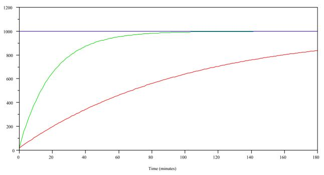
Figure 12 Constant 1000°C Temperature-Time Response in Enclosure and Resulting Element Temperature - Time Relationships
