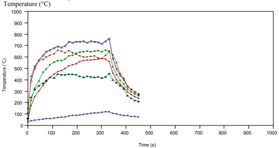
300 mm wide, 1500 mm deep, 300 mm high, wall material = steel, x = 800 mm extra thermocouple 20 mm from floor, ??? mm from rear of enclosure on centreline
