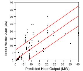
Figure 14 All w/W, Correlation of Equation 6 with Test Data
