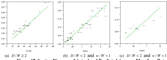
Figure 17 Scatter Diagram of Actual and Predicted Average Mass Loss Rate
