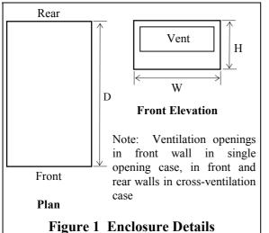
The following terminology and nomenclature is used for the clear internal dimensions of the enclosure (Figure 1):
