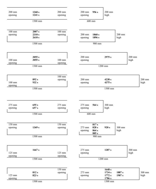
Figure 13 Burnout Times for Enclosures with Openings Both Ends and Similar Enclosures with Single Openings for Comparison
