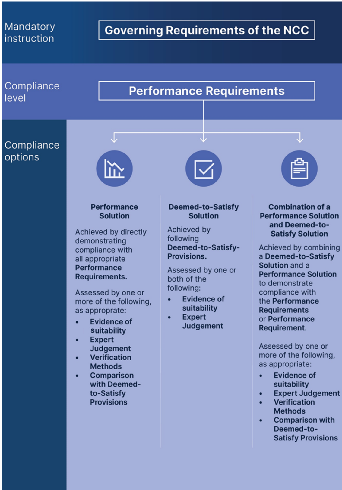
Figure C.1 Demonstrating compliance with the NCC
